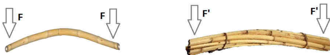
Fig.7: The force to be applied on the bundle of stick (force at each end is F' to bend it and break it finally is much more than the force ( F ) applied on single stick ( F' \gg F )
